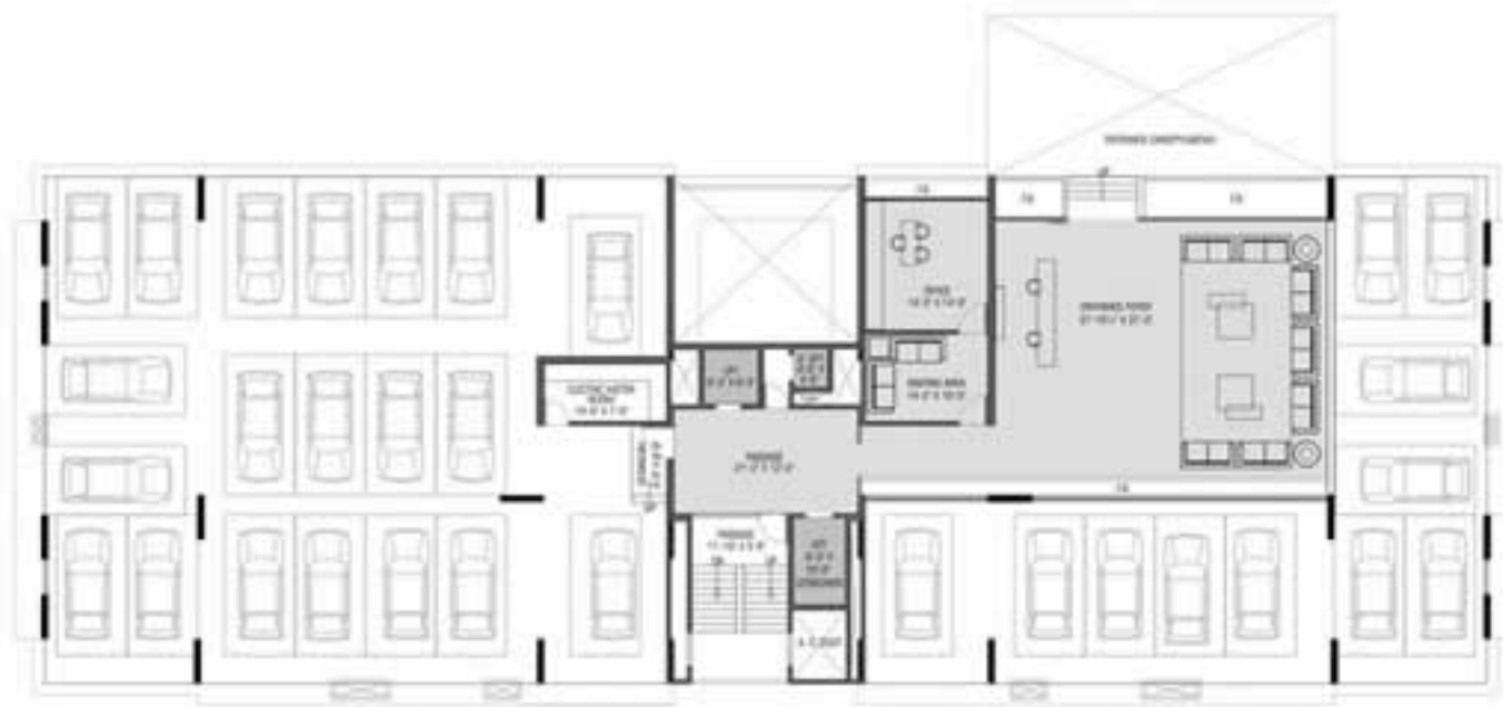
FIRST FLOOR PARKING LAYOUT
